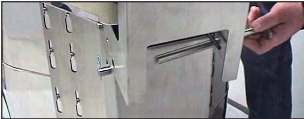
Installing the top-most rod.
