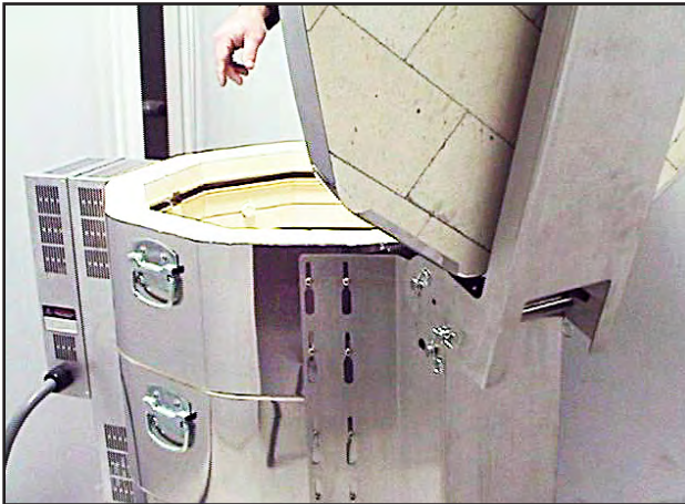
The properly Installed spring hinge open.
