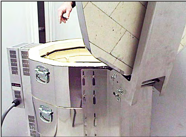
The properly Installed spring hinge open.
