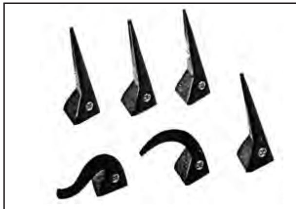
Picture of a "cone pack" (Courtesy of Orton). The ones in the back are before the firing and the ones in the front are after a perfect firing/ These are Self-Supporting Large Cones.
